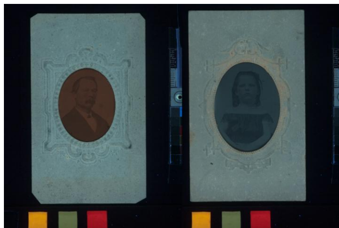
Fig. 5. Two tintypes varnished with a combination of shellac, sandarac and Pinaceae resin. Only the one on the left displays the orange fluorescence commonly expected of shellac.
